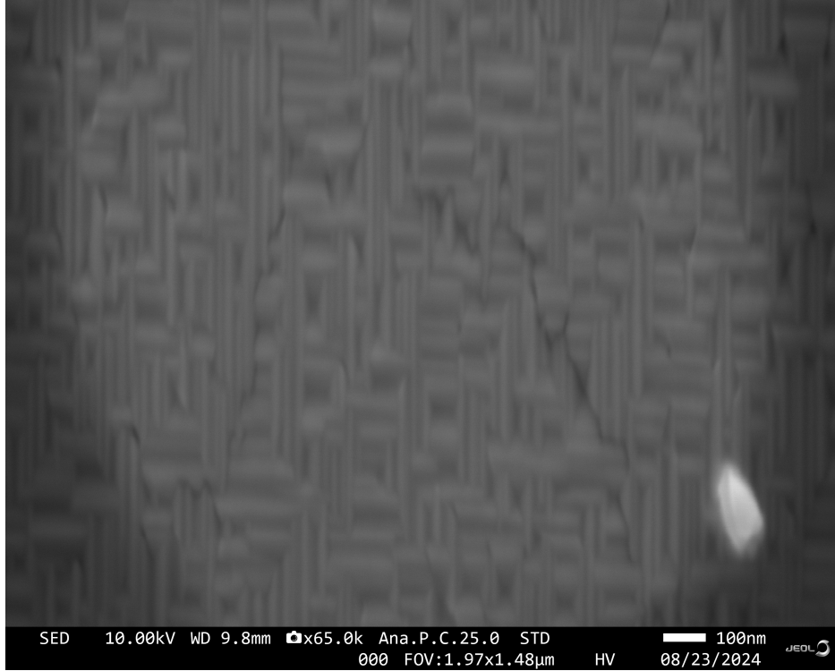
Figure 7.3: SEM image of the surface of a \text{CeO}_2 thin film grown on \text{Si}(001) . We observe a distinctive cross-hatching pattern formed by two domains of \text{CeO}_2 crystallites, with the two domains aligned with the \text{Si}\langle 100 \rangle and \text{Si}\langle 010 \rangle directions.
