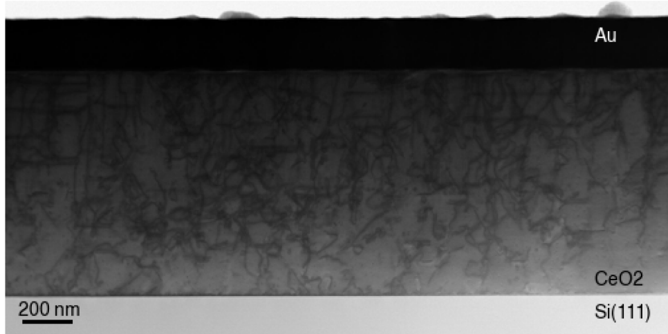
Figure 6.2: Low magnification bright field cross-sectional TEM of the full thickness of an as-grown Er:CeO 2 film (940 nm thick, 3 ppm erbium) on silicon, showing the presence of numerous threading dislocations, with an areal density of approximately 3.3 \times 10^9 dislocations per cm 2 .
